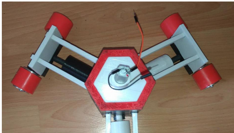
Figure 2. Placing of the DC motor to the robot
